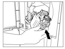
10 Reinstall the stapler unit in its previous position and turn the blue lever 90° to the right to latch the stapler unit.
